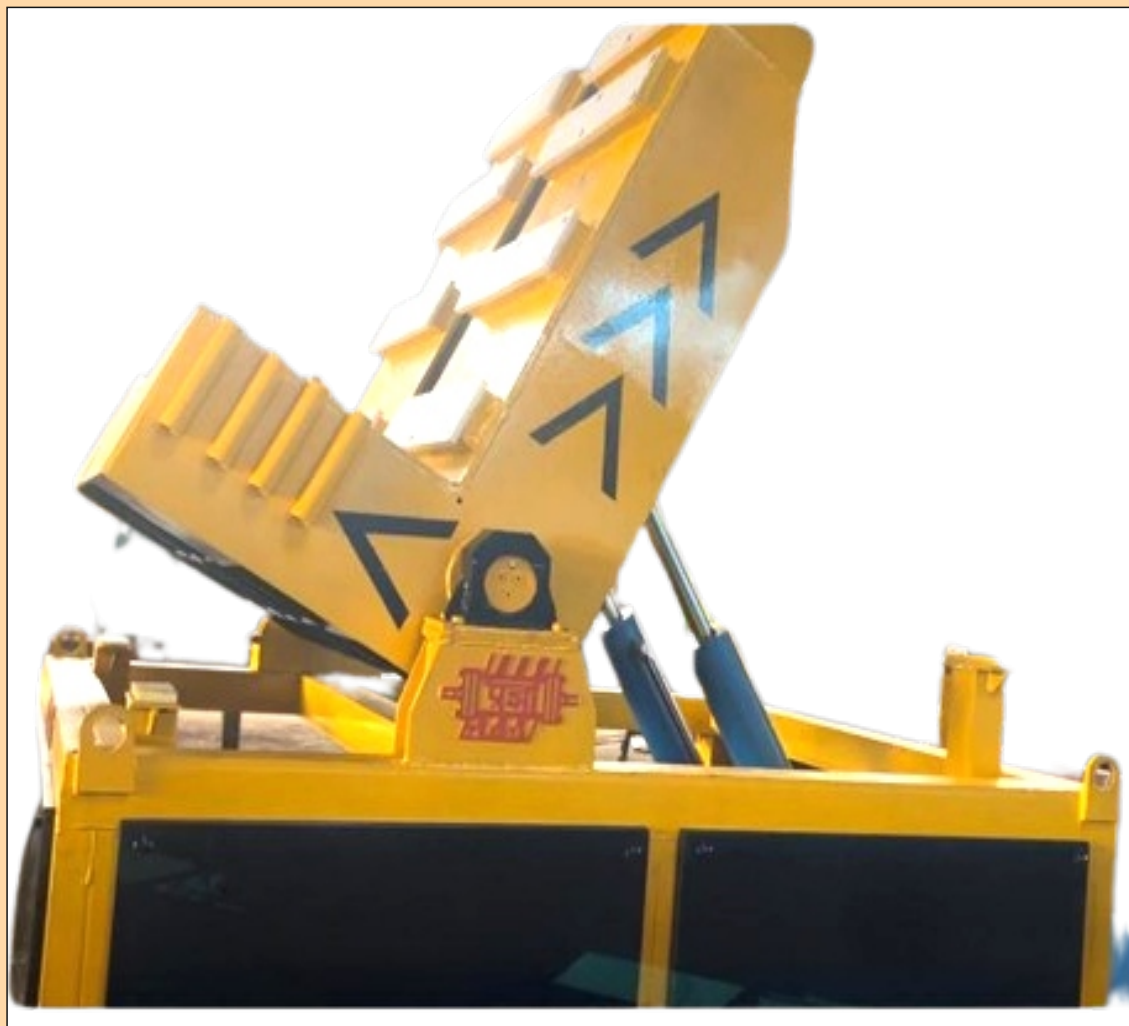
HYDRAULIC COIL FILTER CAPACITY UPTO 45 TON
