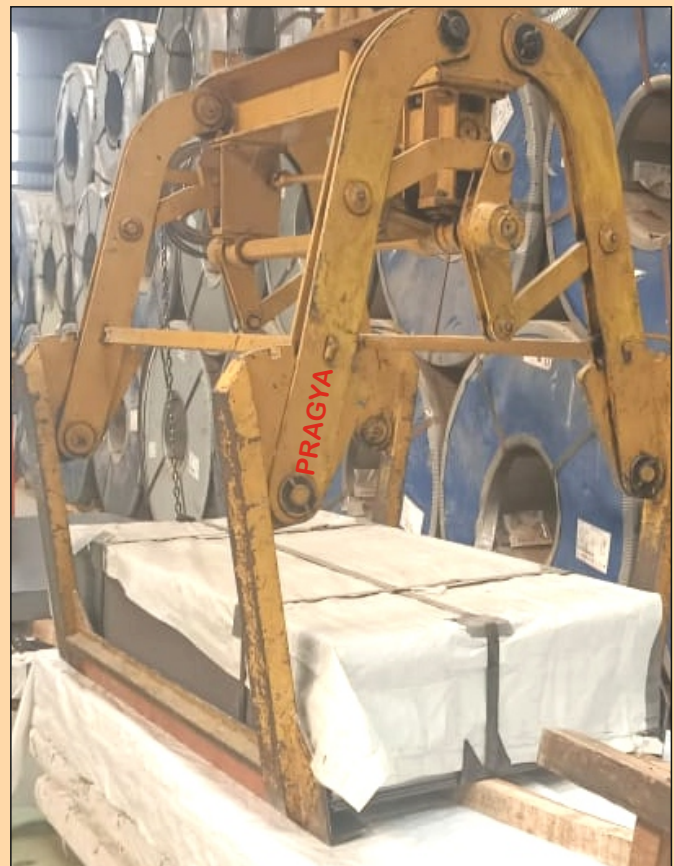
MANUAL TYPE SHEET PACKET LIFTER - 35 METRIC TONS
