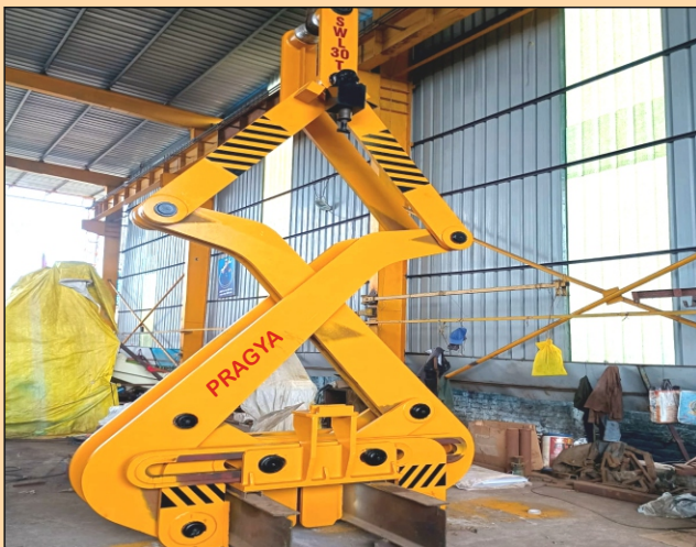
INNER AND OUTER COIL HOLDING GRAB CAPACITY UPTO 45 TON
