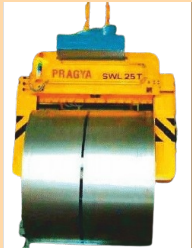
MOTORISED COIL TONG CAPACITY UPTO 45 TON
