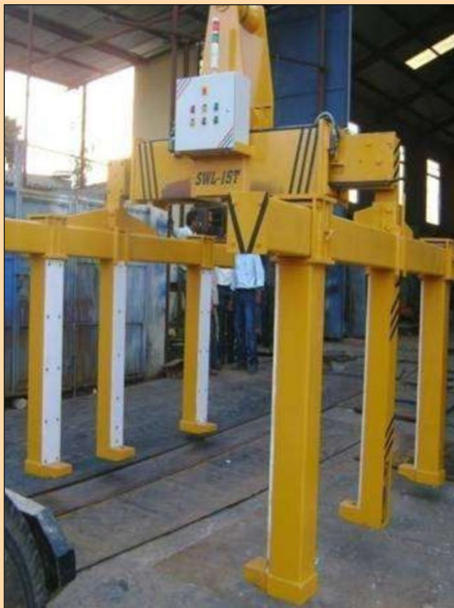
MOTORISED SHEET PACKET / PLATE LIFTER
