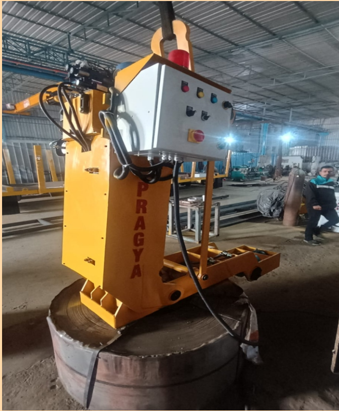
HYDRAULIC AERIAL COIL LIFTER CAPACITY UP TO 15 TON
