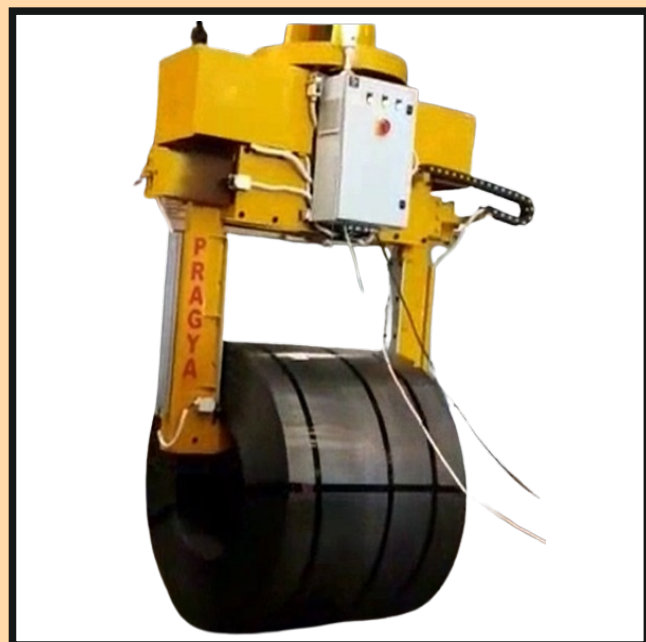
Motorised Coil Tong Upto 45 Tons
