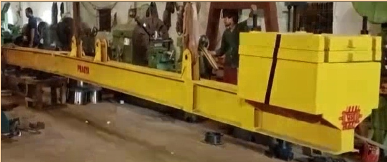
INNER AND OUTER COIL HOLDING GRAB CAPACITY UPTO 45 TON
