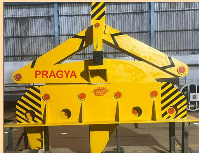
COIL GRAB CAPACITY UPTO 45 TON
