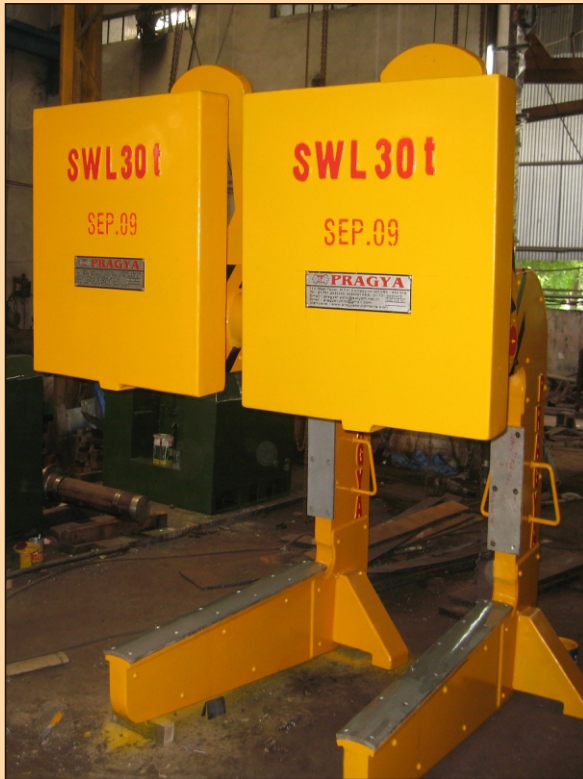
COUNTER WEIGHT C HOOK CAPACITY 5 TON TO 45 TON
