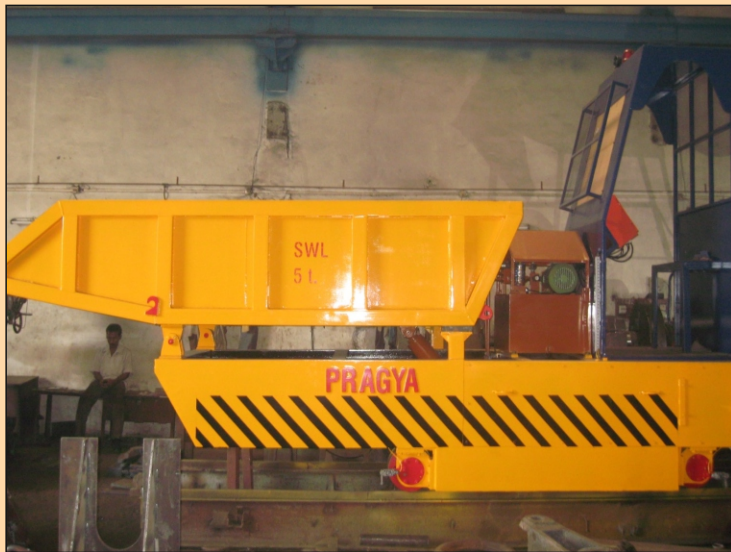
MOTORISED RAIL TRANSFER TROLLEY CAPACITY UPTO 120 TON
