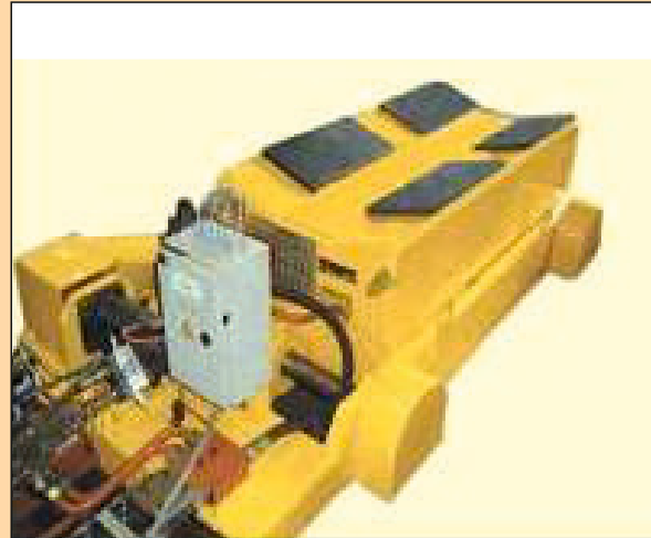
FLOOR TYPE COIL CAR CUM COIL LIFTER (HYDRAULIC)
