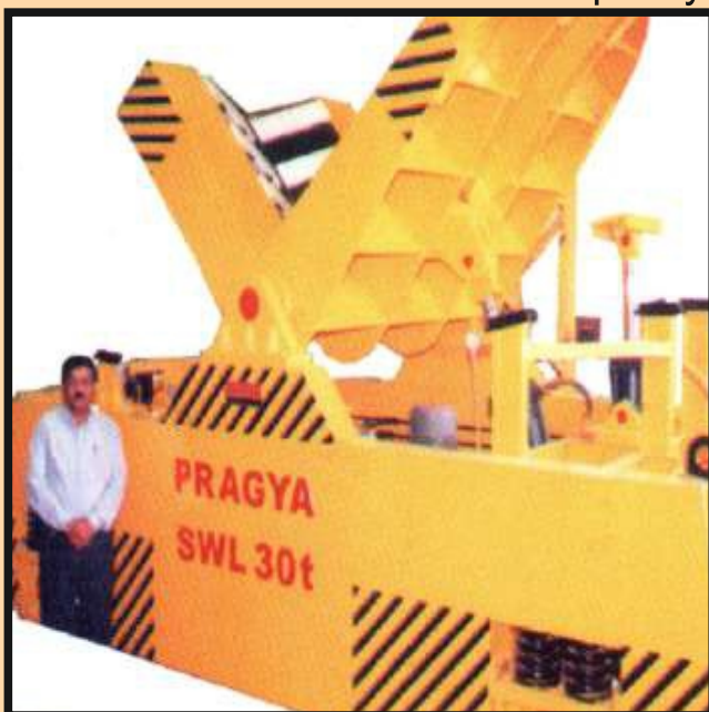
Coil Tilter Cum Trolley up to 70 tons
